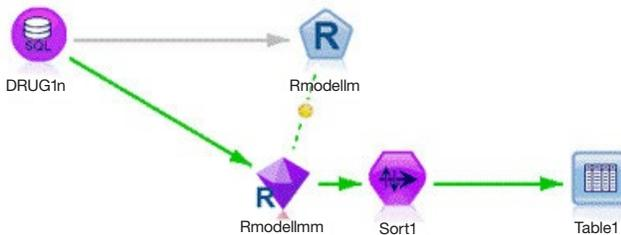
*Figure 3:* IBM SPSS Modeler is used to natively access data in an SQL database with an R model used to score records. Purple indicates that the analytical step is using SQL pushback, which improves performance by executing memory-intensive tasks in the database itself.
